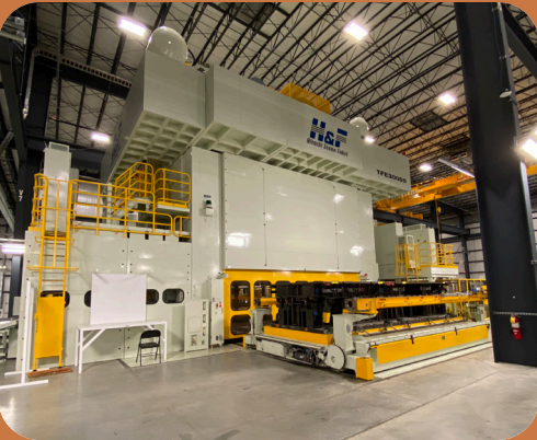
FTIC uses two of these three thousand ton transfer presses to manufacture automotive body structure parts. This press, one of the largest in the industry, is the height of four school buses and the width of three school buses.
